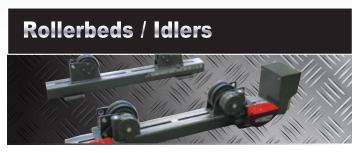
Position the work piece with accuracy or rotation at a constant speed depending on the application.
