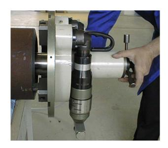
The US 80 is a heavy duty portable pipe beveling tool designed for high quality portable beveling, facing and machining on pipe and tube from 3.5" ID to 14" OD (80 to 360 mm). Each standard tool plate accepts multiple tool bits allowing up to four simultaneous machining operations. Such operations may include beveling, facing, counterboring, compound beveling and OD chamfering on heavy wall materials.
