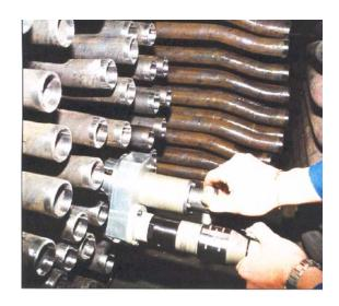
The US 40 CH with its reduced overall dimensions and its lightweight is specially designed for applications that have limited clearance requirements such as boilers.
