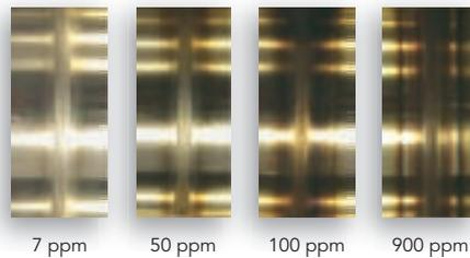
result. Oxidation develops through contact with oxygen when the material is heated to welding temperature. After welding has ended it is important to maintain the inert atmosphere until the temperature of the work-piece is below 250°C, depending on the material. These Schnorrer advanced gas purge systems are under continuous development to meet many demanding technical specifications and functional needs, and to meet these needs economically.
