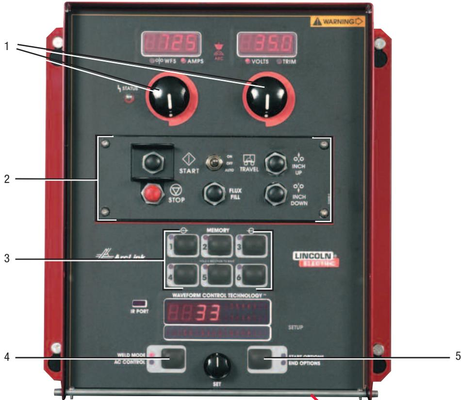
1. Two **control knobs** can increase or decrease Wire Feed Speed (WFS), Voltage, and Amps. Any of these adjustments can be made “on-the-fly”.
