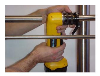
The portable machine SE 25 RA is specially designed for facing in position the diameters from 2 mm to 25,4 mm **under tight places of work**.
