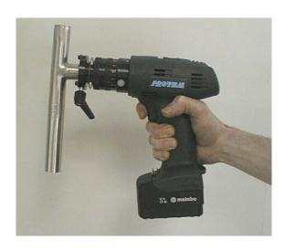
The portable machine SE 25 is specially designed for facing in position the diameters from 2 mm to 25,4 mm OD.
