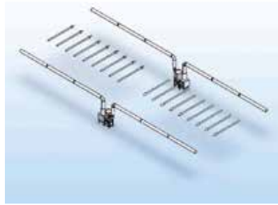
Double-parallel push/pull-system with 2 filter units and fans.
