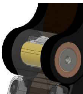
Axial spring-loaded system: to account for tube "out of round"
