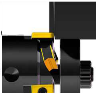
J bevel with profile guide roller
