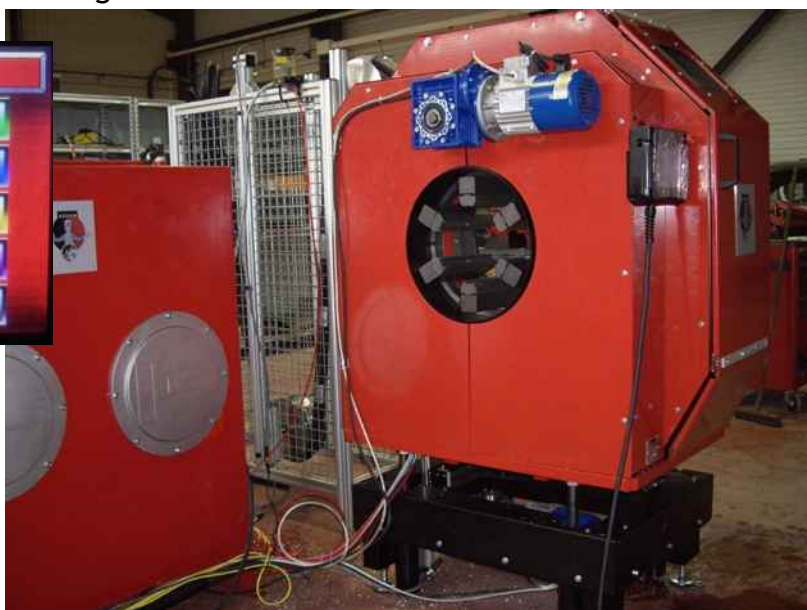
Carbide orbital cutting (hydraulic motor)
