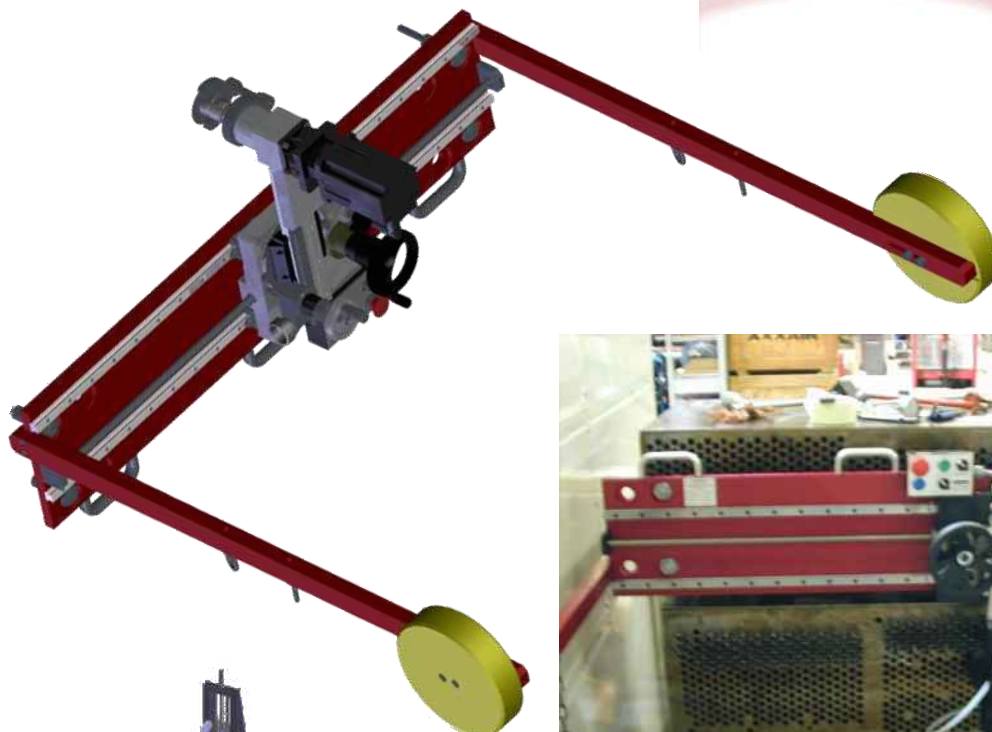
Tube cutting on plate
