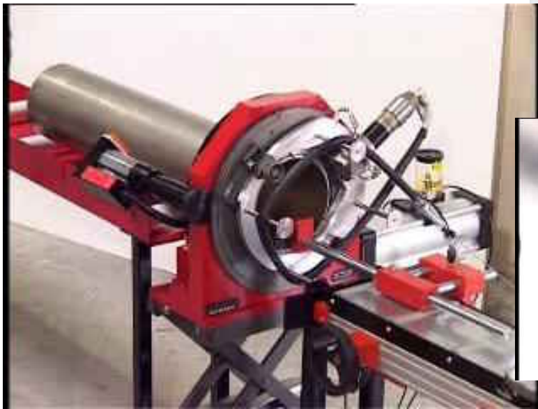
Orbital cutting of large-diameter, thin titanium
